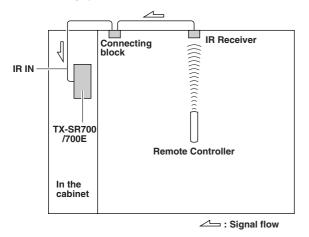
The IR IN input allows you to control the TX-SR700/700E from the remote zone (Zone 2) with the remote controller even though the remote zone may be on the other side of the building from the main zone. The diagram below shows how to make the proper connections for the remote zone.
